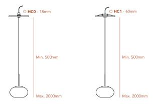
HCO - Recommended for houses with access above the plasterboard ceiling.HC1 - Recommended for houses with NO access above the plasterboard ceiling.
