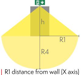
R1 distance from wall (X axis) R4 distance from wall (Y axis) TWS3092WME
